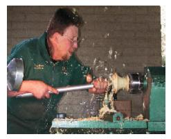
5. With the ball in the jam chuck, the underside of the ladle is turned and finished. This operation takes a very delicate touch since a catch would send the piece flying across the room. Less talented turners might be able to cut the underside of the ladle on a band saw before starting on the ball. 6. Finally, with the ball in the chuck and the handle flying precipitously around in space, the top of the bowl is faced off and the bowl is hollowed out.
