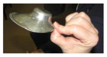
He then set up another blank and proceeded to go through the process with step by step commentary. Here he is centering the blank.
