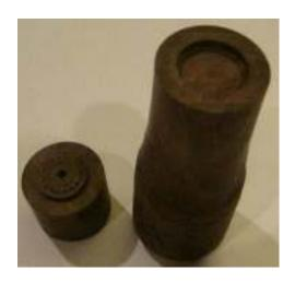
True the OD if needed and make a  $1/16 \times 1/16$  tenon on the end of the piece. Now hollow out a semi-spherical bowl about 3/4 to 7/8 deep in the end, leaving a 3/32 to 1/8 wall at the rim.
