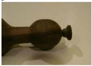
Reinstall the chuck on the lathe and support the piece with the live center. Sand the rattle to final grit and then make 3 small V cuts about 3/16 apart to guide the wire when burning (the middle v is on the glue line). Burn the 3 lines with a wire. Pull the tailstock back and carefully remove the nub from the end of the piece. Sand as required to remove any tool marks.
