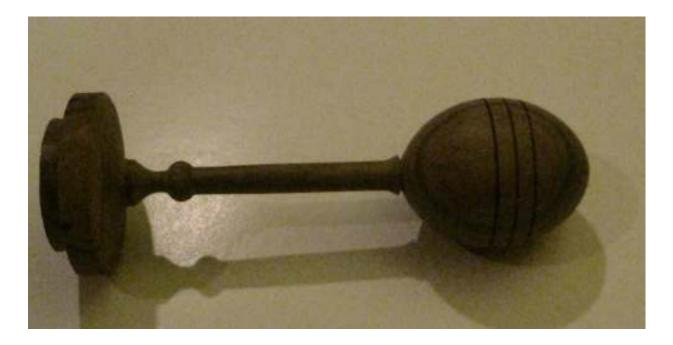
Finish cutting the bead end off of the waste stock. Clean up the end of the handle and sand by hand to remove the last little bit.
