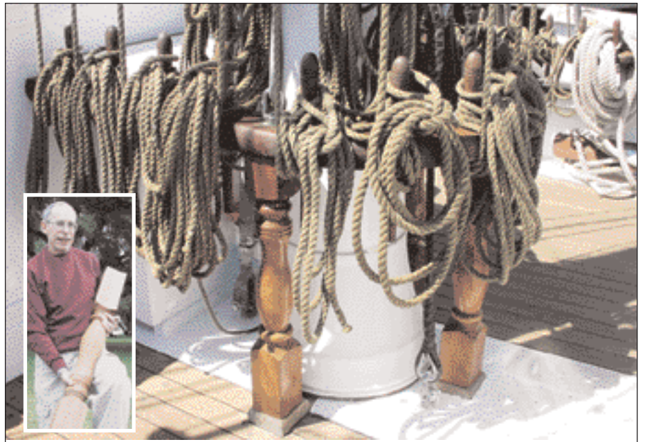
Damon Siples, insert, holds one of the ten 48"-tall fife rail stanchions he turned from purpleheart. The larger photo shows two of the stanchions in use.
