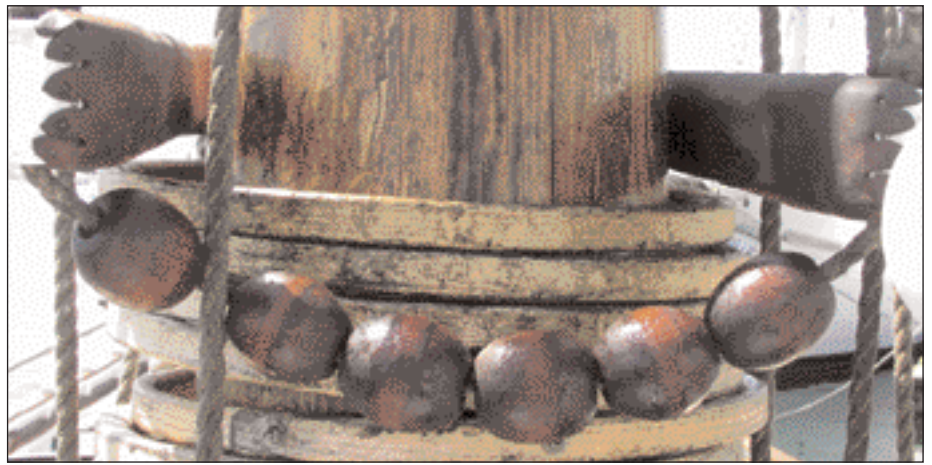
Parrell beads, turned from courbaril, are shown on the main gaff throat. The beads permit the gaff to travel up and down the main mast.
